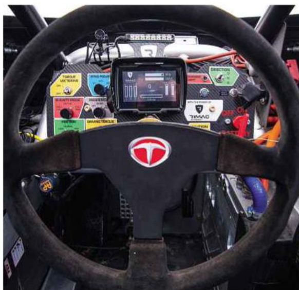
Left: a lot to take in: the eRunner's fascia is awash with switches and buttons. Right: spaceframe chassis is the work of Monster Sport; battery packs reside either side of the driver's seat
